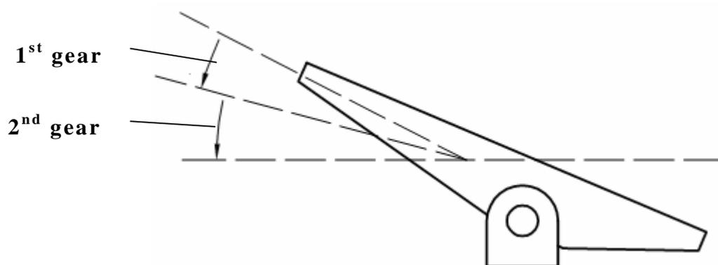
**Treadle Pedal Schematic Diagram**
