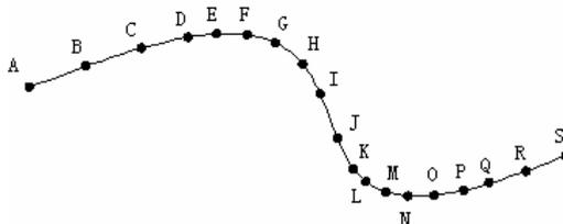
2. Lower the needle by handwheel, and stop when it almost contacts template. Use Arrow Key to move machine needle from origin to point A, with operation panel shown as Fig. 6-10 in moving process. And [K001] displayed on menu
