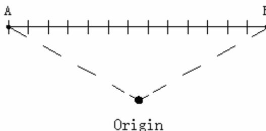
2. Lower the needle by handwheel, and stop when it almost contacts “origin” position in the template. Use arrow key to move machine needle from origin to point A, with operation panel shown as Fig. 6-14 in moving process. And [K001] displayed on menu display indicates the key point. After moving to point A, press
