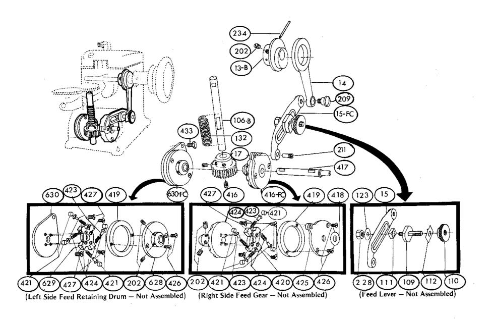
ILLUSTRATED IN SHADOW MACHINE—GEAR AND FEED
