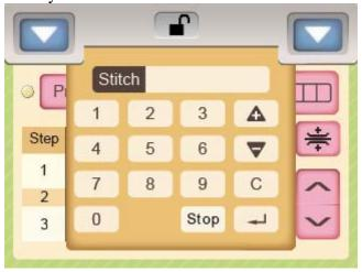
Step 8. Enter the required the number of stitches, press Stop to display the number of stitches and additional 's' that machine stops immediately when the setting stitches are completed and the next sewing Step can start to run by toeing down the pedal unless the pedal returns to neutral position in advance.
