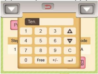
Step 3. Enter the required tension value. Then press the \_\_\_\_ to save the value and to close the keyboard.
