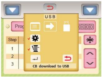
Step 5. Press to pop up the dialog box menu as shown. Press "YES" to download the parameter settings and Program data from MCU to the USB flash drive. The parameter file "TCPARAME.TCD" and the Program data file "TCPROCES.TCD" will be stored in the root directory of the USB flash drive.
