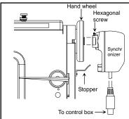
Mounting the Synchronizer onto the flange of hand wheel and match the stop groove of the
